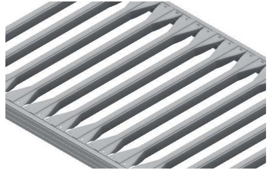
12 Lightened secondary beams *
